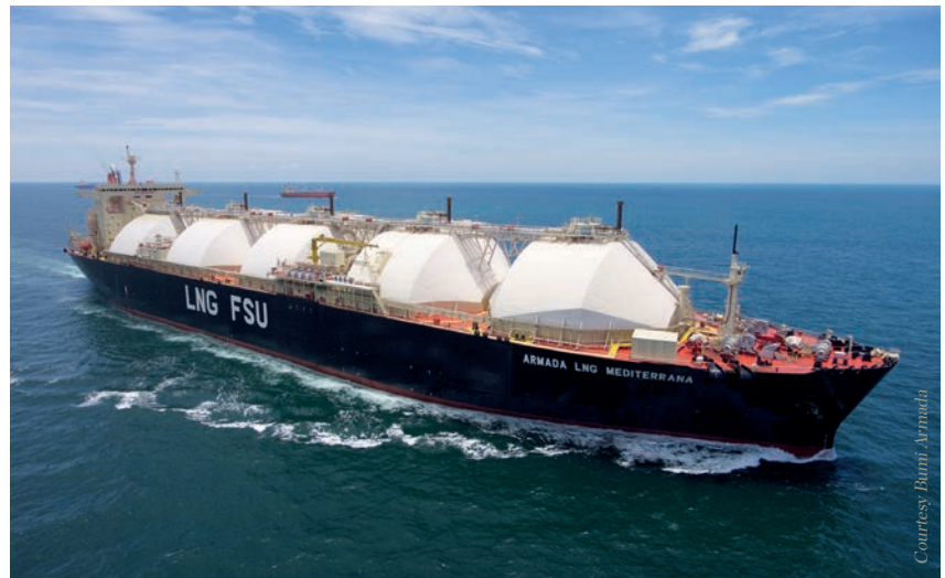
Armada LNG Mediterrana, originally an LNGC built in 1985 with MOSS tanks – converted into an FSU ready for operation in Malta in 2016.
